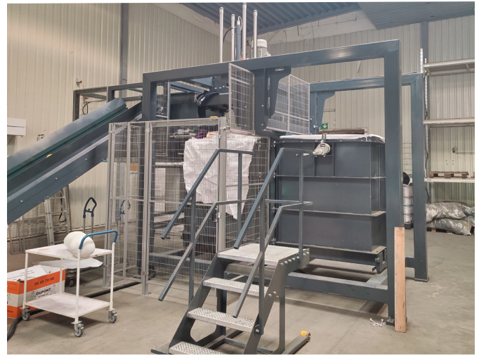
The new pressing machine, which presses all the textile waste at our warehouse.
